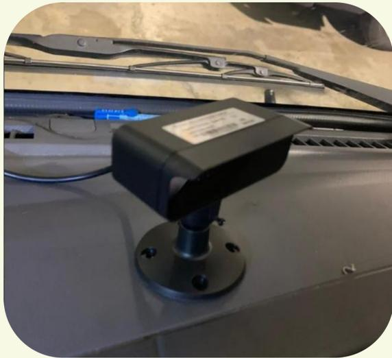
ADAS – Sensors installed on vehicle to provide alerts for collision avoidance
