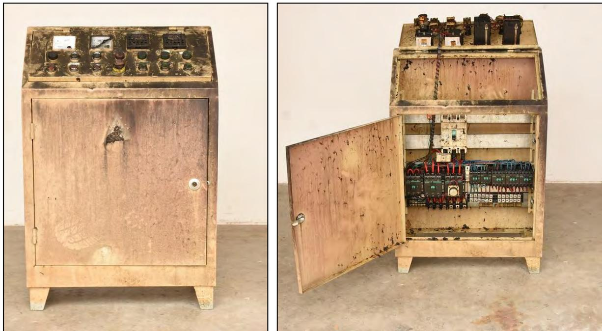
**Figure 34:** As-received condition of the electrical panel.
