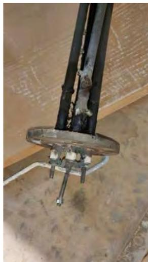
39. The damaged heater was replaced with a new spare heater that morning. Later that afternoon, the Mixer Machine was operated again to make fire clay.
