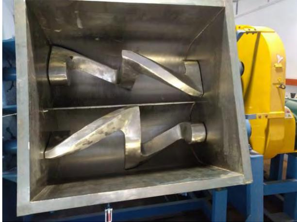
17. When tilted, the Front Pipe would have to be closed to prevent oil in the oil jacket flowing out. The Mixer Machine was delivered with 1 end cap placed on the Front Pipe.
