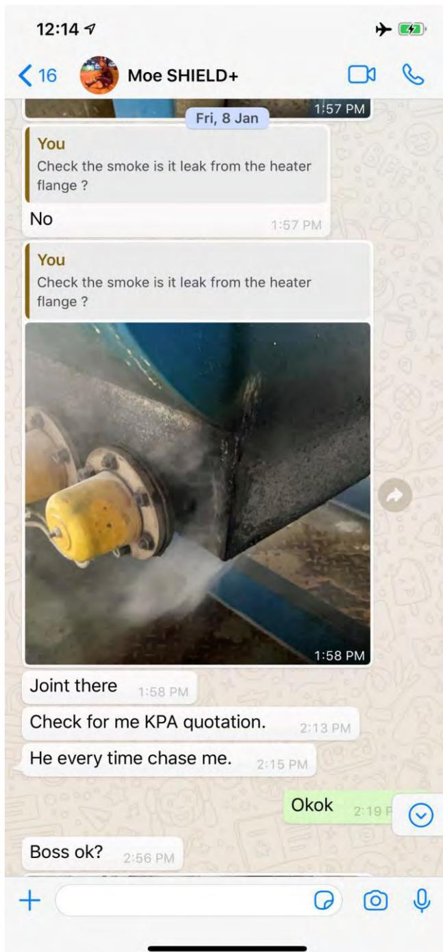
63. The IC will hear from Moe that, from that time until the next incident on 12 February 2021 (see [65] below), white smoke came out from the bottom corners of the oil jacket in the last 10 minutes of the operation of the heaters whenever the Mixer Machine was used to make fire clay.
