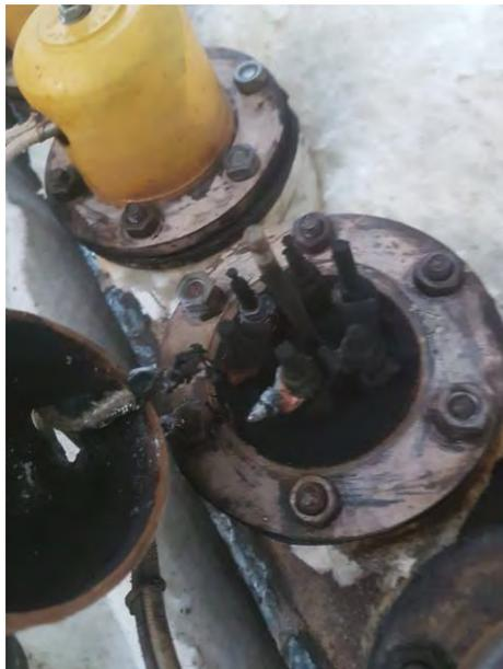
75. Moe forwarded the photos to Mr Chua at 9:21am **[S-32]**. Further photos of the damaged / burned Heater No. 2 were also sent by Marimuthu to Chua:
